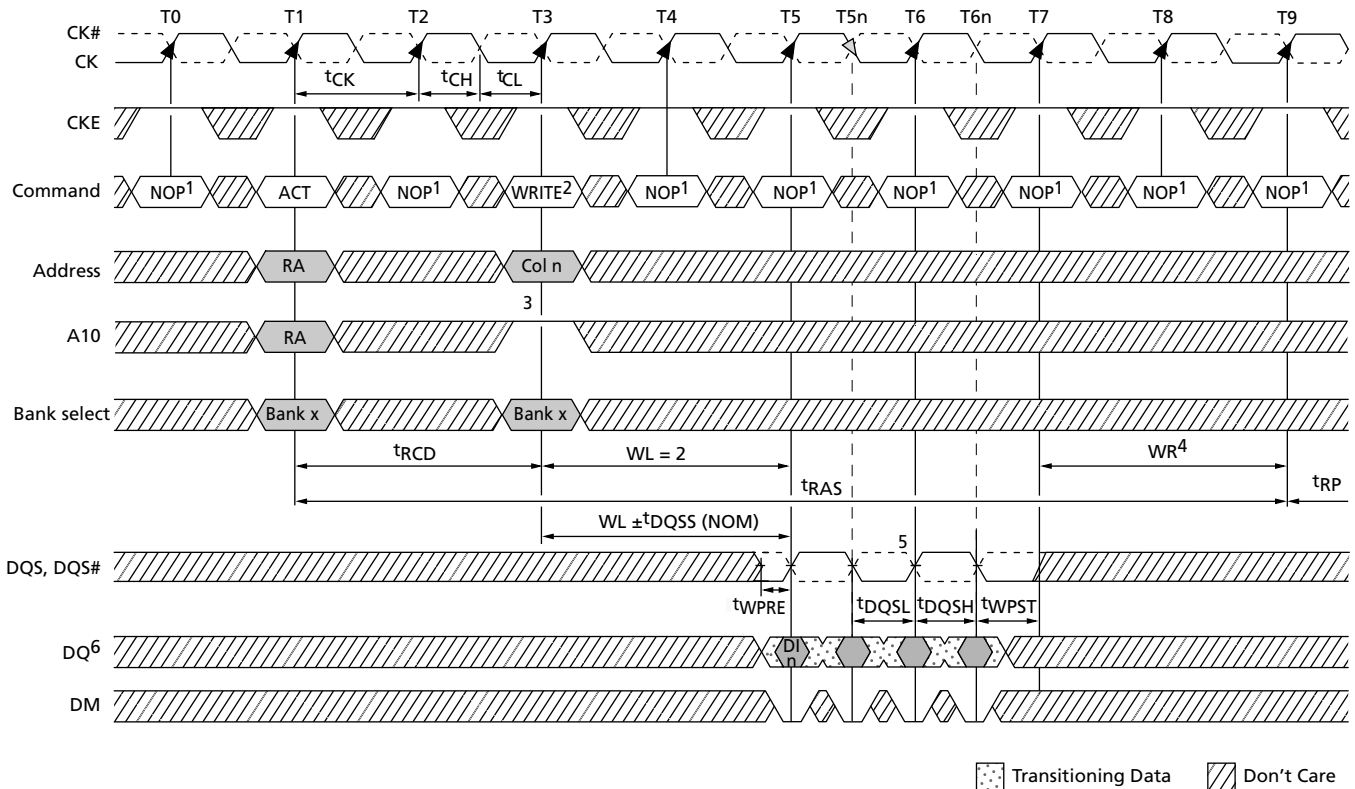
Figure 65: Bank Write – with Auto Precharge
